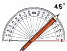
**Step 5:** With the protractor or a ruler draw a straight line from A to the mark you just made. Label this point C.
