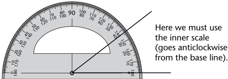
You can also place the protractor on the angle using the other arm. Then the correct position looks like this:
