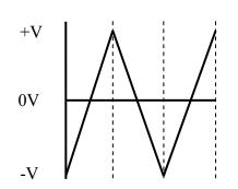
Output must show Triangular waveform√ +√√ -V ✓
