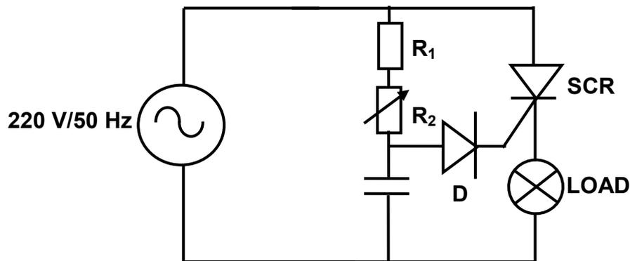
**FIGURE 6.2: LAMP-DIMMING CIRCUIT**
