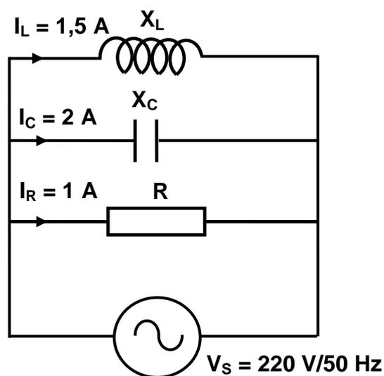
FIGURE 5.1: PARALLEL RLC CIRCUIT
