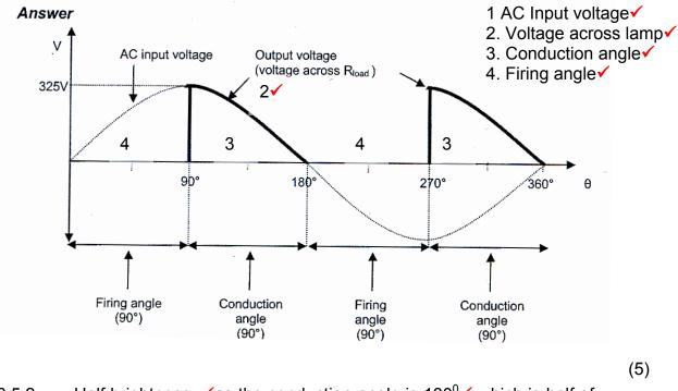
6.5.2 Half brightness, ✓as the conduction angle is 180<sup>0</sup> ✓ which is half of 360<sup>0</sup> therfore half power. ✓ (3)
