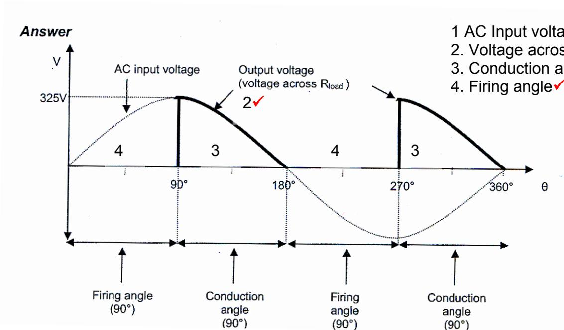
6.5.2 Half brightness, ✓ as the conduction angle is  $180^{\circ}$  ✓ which is half of  $360^{\circ}$  therefore half power. ✓
